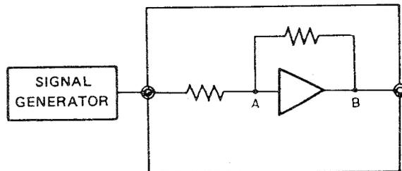
Figure 6— Negative Feedback Amplifier Gain Measurement.
